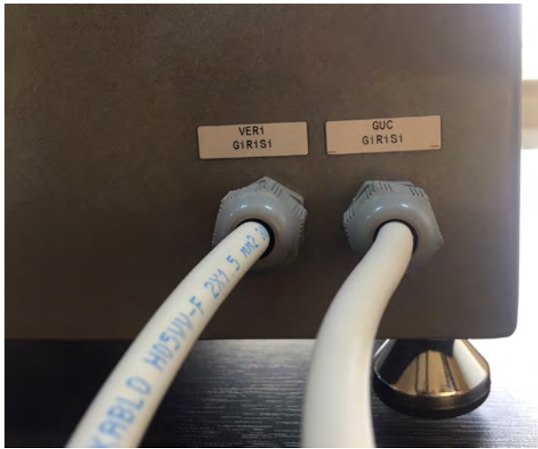
Data Input (Flow meter etc.) - Power Input
